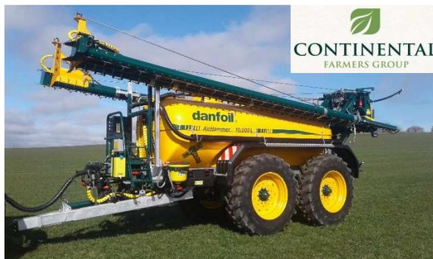
*"It is by far the most efficient sprayer on the farm."* Says Esben Nielsen. With it's 36m span and 10.000 L tank. It takes 10 hours to do the 260 Ha. Including filling, transport and application
