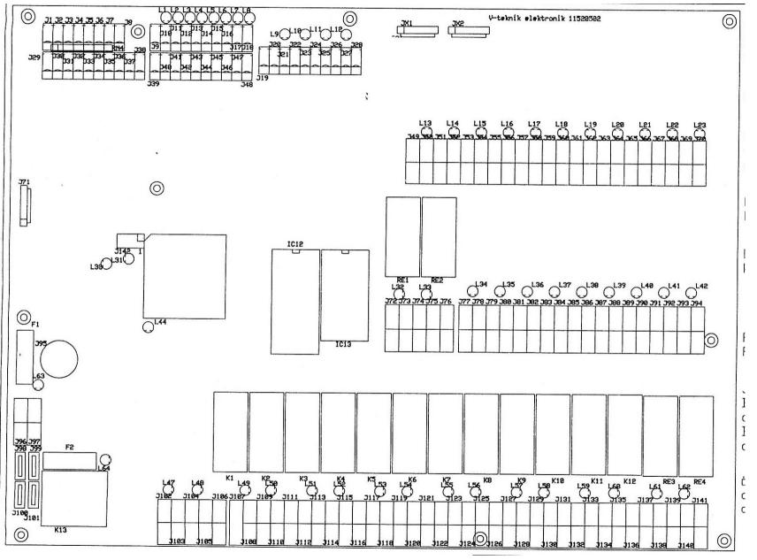
L30 Indicates reset lights up shortly at high voltage
