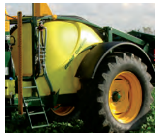
Clean water in the tank The idea behind the injection system is to add the chemicals separately, so you only have clean water in the tank, and therefore maximum flexibility whilst spraying
