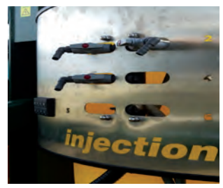
Calibration The injections system requires calibration depending on different types of chemicals. With the danfoil injection system, this is easily operated on the sprayer.
