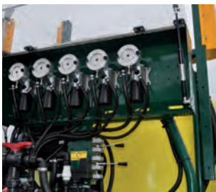
Injections system From 1 to 5 pumps.
