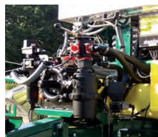
Pump for agitation of the tank (extra equipment) An extra pump for agitation can be mounted in the main tank, which secures further flexibility, as this makes it possible to add chemicals directly in the main tank.
