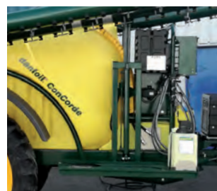
Cleaning system Automatic cleaning system with a separate cleaning tank, secures both a clean system, and no mix of different chemicals
